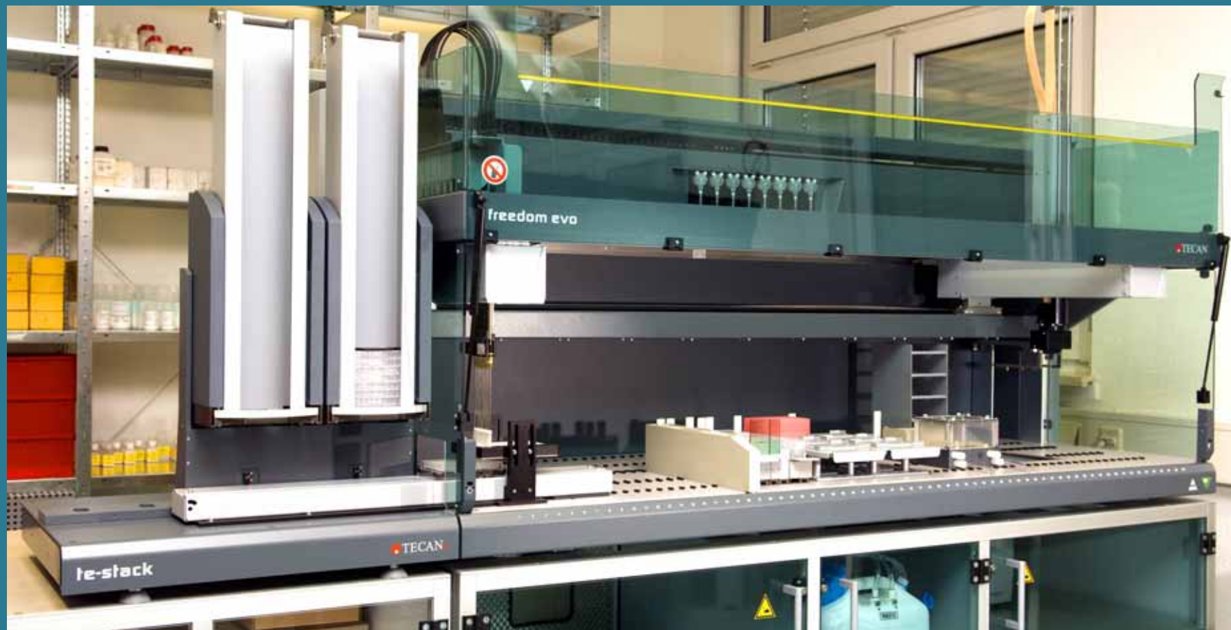
Tecan Freedom Evo Pipetting Robot Configured As Chromatography Workstation
